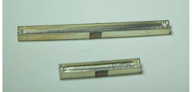
Fig. 1. Manufactured 22 mm and 44 mm long WR10 waveguide submounts
